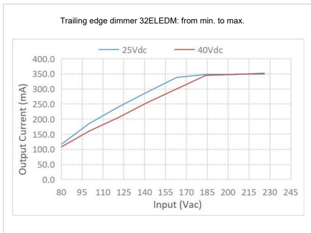
Trailing Edge Dimmer 32ELEDM: Minimum to Maximum Dimming Curve
