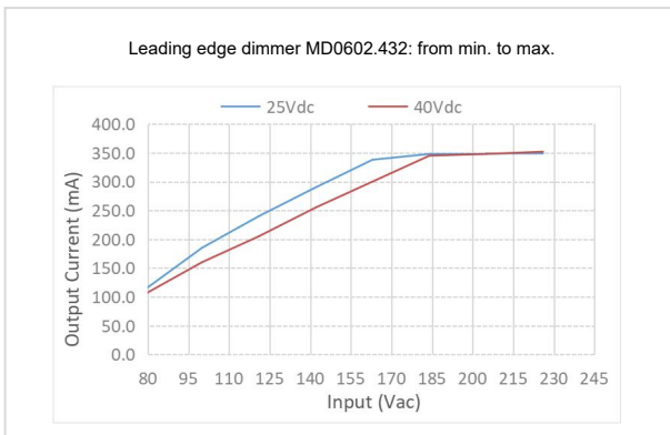
Leading Edge Dimmer MD0602.432: Minimum to Maximum Dimming Curve
