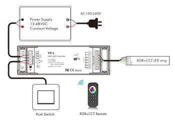
Note: Long press match key for 10s, RGB and CCT light can not be on at the same time. Long press match key for 15s, RGB and CCT light can be on at the same time. above operation will also restore the factory setting.
