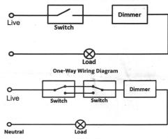
**Two-way Wiring Diagram**
