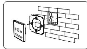
Fix the panel dimmer base on the bottom case with screw.
