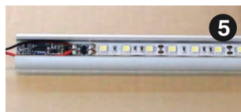
5 Solder the LED strip to the output terminals of the module
