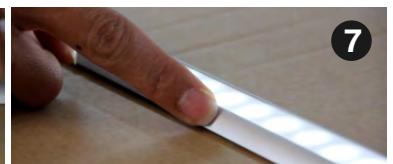
7 Touch the aluminium profile to test functionality
