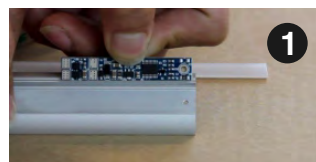
1 Drill a 1.5mm hole in the aluminium profile and screw the profile in place
