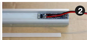
2 Solder the input power wires to the input terminals of the module
