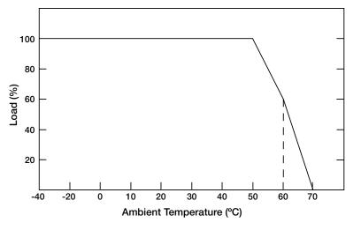
If being used in higher ambient temperatures, ensure the load on the LED driver is de-rated in accordance with this chart. Failure to do so could lead to a premature failure, which is not covered by the warranty.
